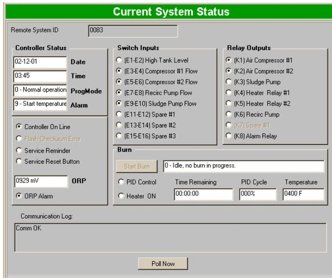
Figure 3. Current Status of the EnviroServer 600 Installed at the Ventura Sanitation District.
