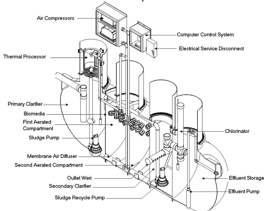
Figure 1. Schematic of EnviroServer Advanced Wastewater Treatment System.
