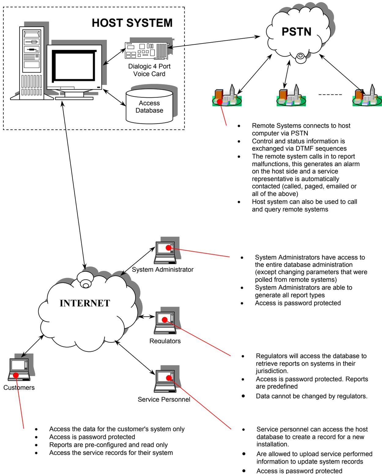
Figure 2. Illustration of the Systems Functionality and Access.
