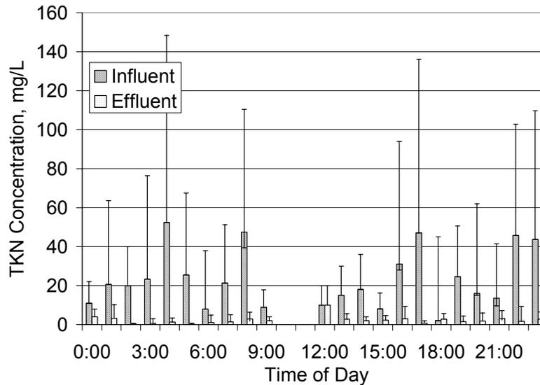
**Figure 8. Hourly influent and effluent TKN concentrations for weekday track study. Error bars show maximum and minimum values. (N=4)**
