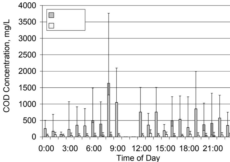
**Figure 7. Hourly influent and effluent COD concentrations for weekday track study. Error bars show maximum and minimum values. (N=4)**
