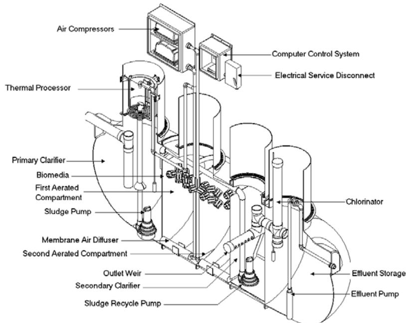
**Figure 2. Schematic rendering of an Enviroserver 600 residential treatment system.**
