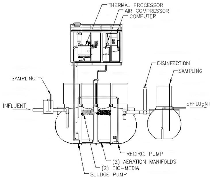
**Figure 1. Schematic rendering of the UCR test facility, an Enviroserver 600 residential treatment unit with an above ground thermal processor and a separate chlorination tank.**
