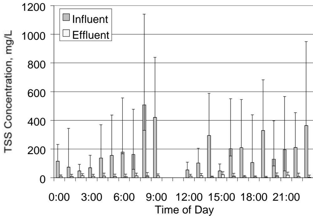
Figure 8. Hourly influent and effluent TSS concentrations for weekday track study. Error bars show maximum and minimum values. (N=4)
