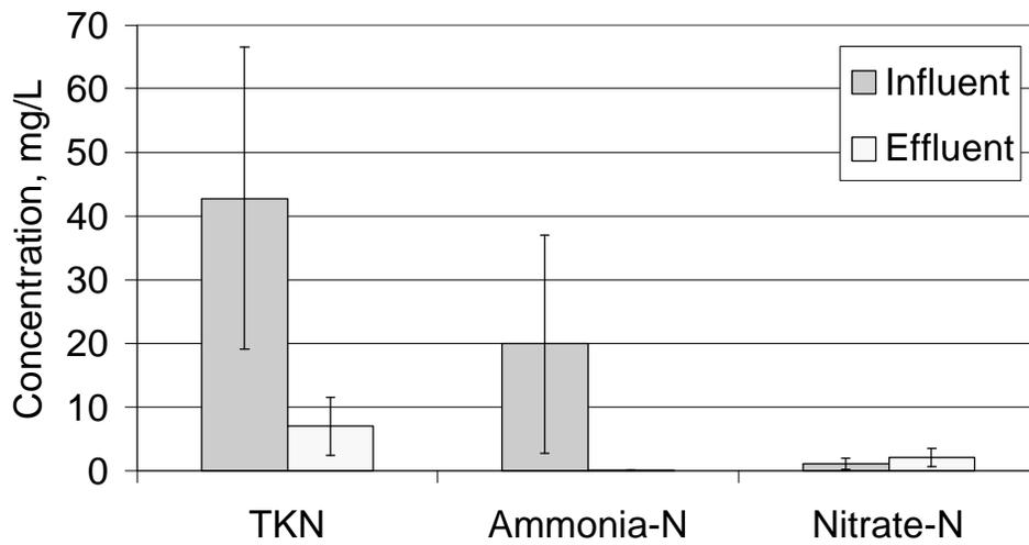
Figure 5. Average influent and effluent TKN, Ammonia-N, and Nitrate-N concentrations. Error bars show one standard deviation. (N=24 for TKN, and N=31 for NH<sub>3</sub> and NO<sub>3</sub>)
