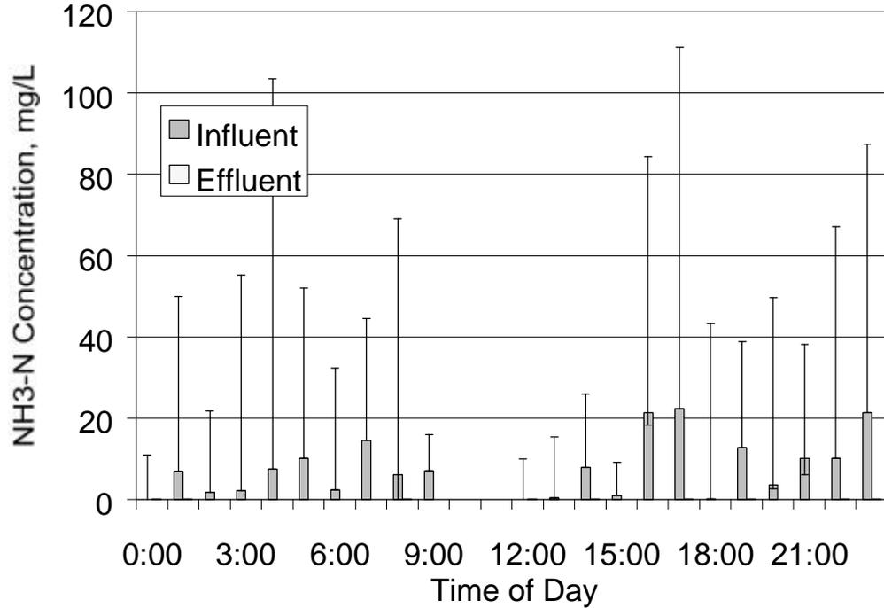
Figure 10. Hourly influent and effluent Ammonia-N concentrations for weekday track study. Error bars show maximum and minimum values. Note, maximum concentration was 0.1 mg/L in effluent. (N=4)
