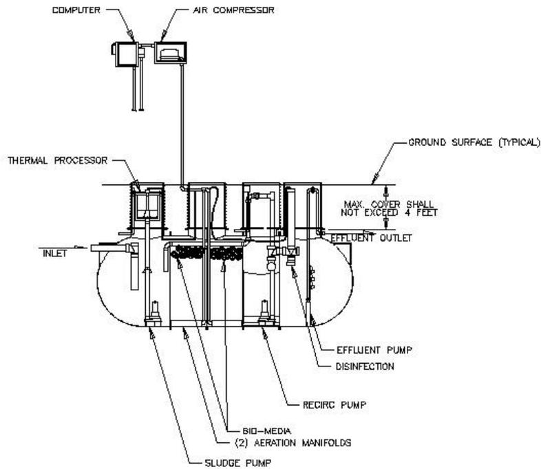
Figure 1b. Schematic rendering of the commercial EnviroServer 600 residential treatment unit.
