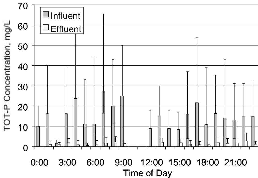
Figure 11. Hourly influent and effluent Total-P concentrations for weekday track study. Error bars show maximum and minimum values. (N=4)
