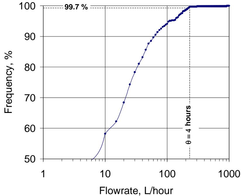
Figure 3. Frequency distribution of hourly flowrates. The hydraulic residence time in a compartment having a volume of 950 L (250 gal) exceeded 4 hours for 99.7 % of the time during the evaluation period.
