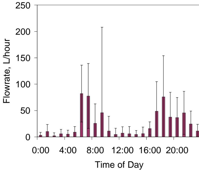
Figure 2. Average hourly flowrates with error bars showing one standard deviation.
