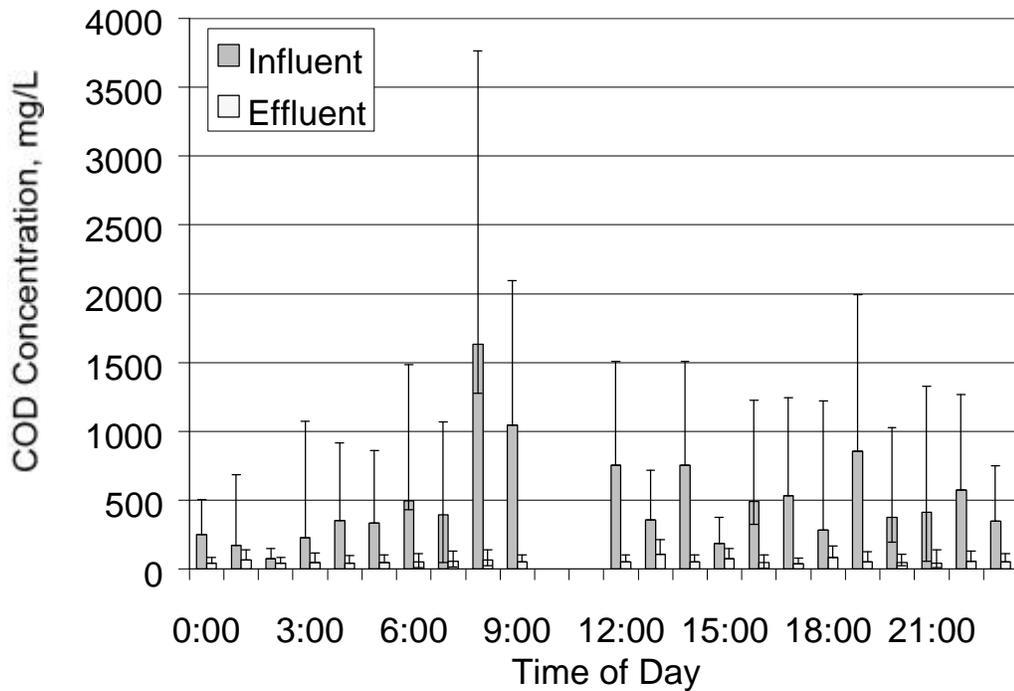
Figure 7. Hourly influent and effluent COD concentrations for weekday track study. Error bars show maximum and minimum values. (N=4)
