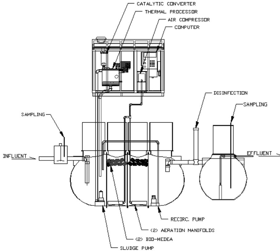
Figure 1a. Schematic rendering of the UCR test facility, an Enviroserver 600 residential treatment unit with separate chlorination tank.
