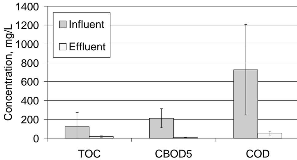
Figure 4. Average influent and effluent TOC, BOD<sub>5</sub>, and COD concentrations. Error bars show one standard deviation. (N=31)
