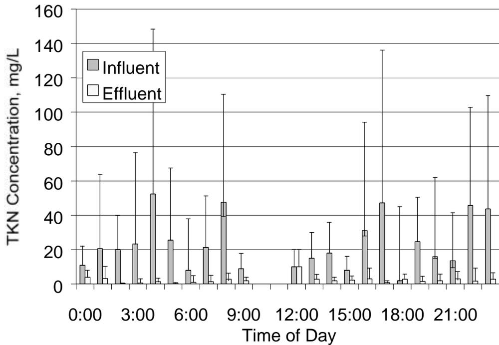
Figure 9. Hourly influent and effluent TKN concentrations for weekday track study. Error bars show maximum and minimum values. (N=4)
