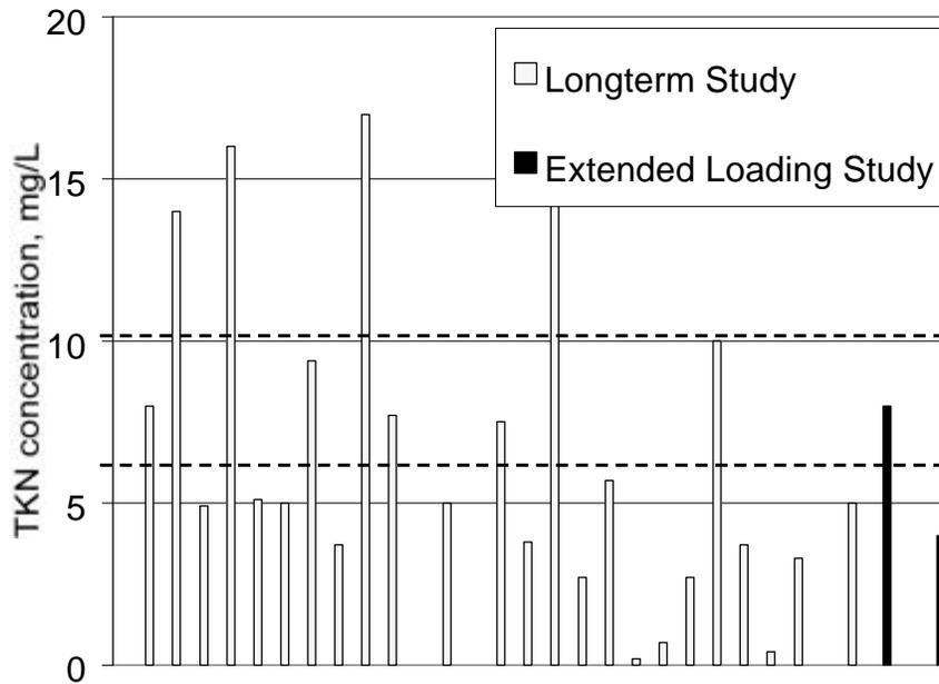
Figure 13. Effluent TKN concentration for longterm evaluation study (normal loading) and for extended loading rates of 135%, 160% and 173% based on a nominal daily wastewater flow of 600 L/day. Dotted lines represent average and average plus one standard deviation of effluent TKN concentrations for the Longterm Evaluation Study.
