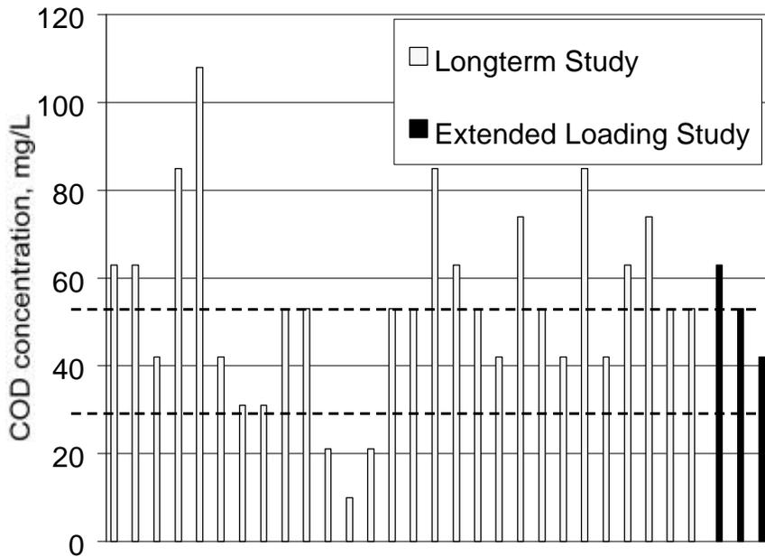
Figure 12. Effluent COD concentration for longterm evaluation study (normal loading) and for extended loading rates of 135%, 160% and 173% based on a nominal daily wastewater flow of 600 L/day. Dotted lines represent average and average plus one standard deviation for effluent COD concentrations for the Longterm Evaluation Study.
